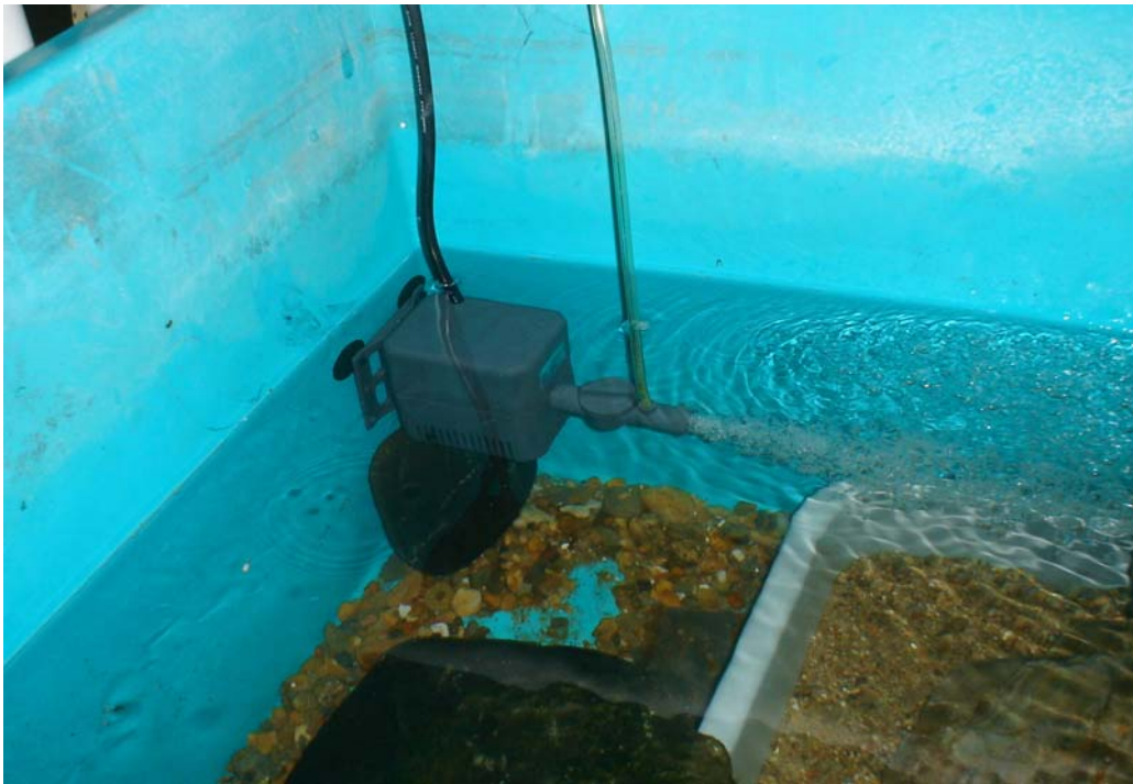
Figure 12: Powerhead being used to create circulation.
